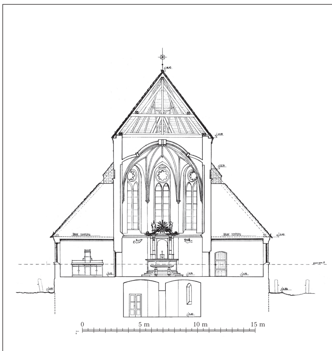
Figure 6. Kochanówka, Church of St. Lawrence: A — cross-section of the nave. Measurements performed by the Faculty of Architecture, Warsaw University of Technology; Gabriela Zielińska and Jan Stusio, 2021, ZAP WAPW Collection ref. no. 3850; B — cross-section of the chancel. Measurements performed by the Faculty of Architecture, Warsaw University of Technology; Zofia Pabiańczyk and Agata Stefańska, 2021, ZAP WAPW Collection ref. no. 3849
